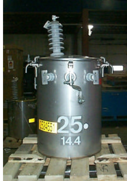
Stainless Steel Transformer
